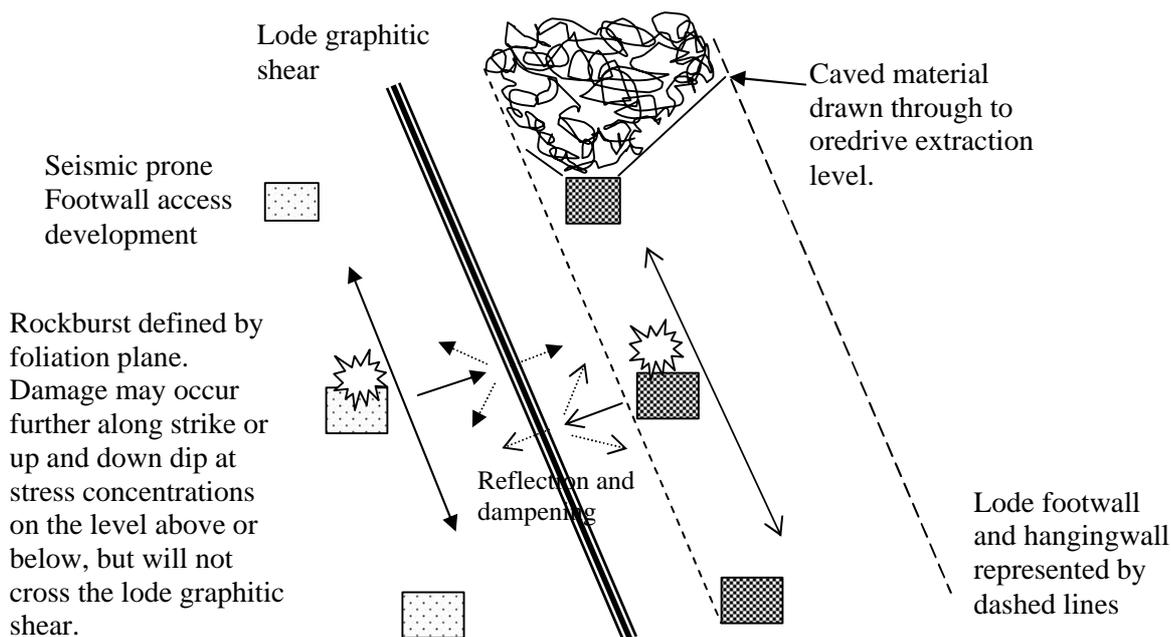
Figure 2: View in cross section showing damage transmission from rockbursts.
