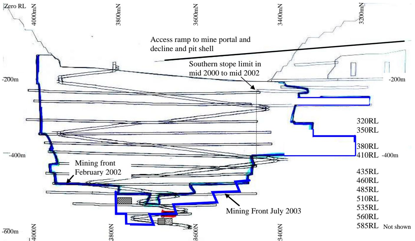
Figure 4: Change in mining front with major rockburst locations from February 2002 to July 2003
