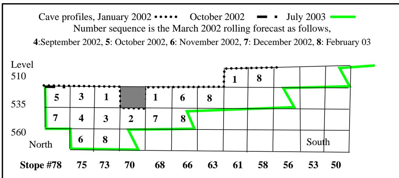
Figure 5: Sequence of stope extraction to achieve good mining front angles from
