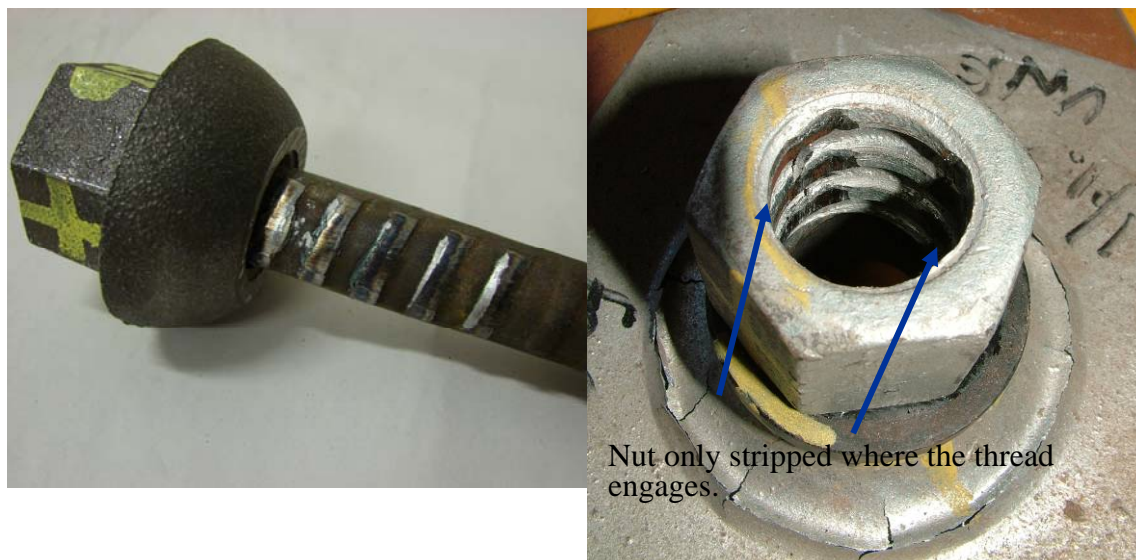
Figure 11. Shearing of the thread on the bar and mine nut.
