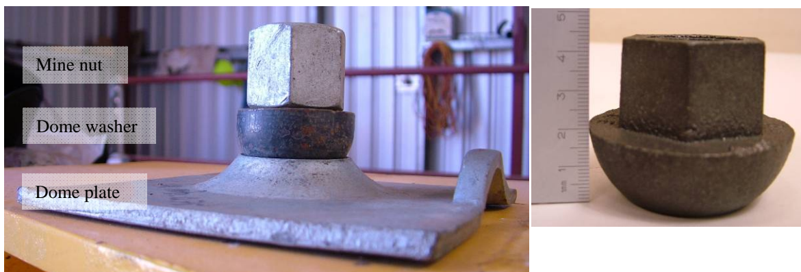
Figure 5. Surface hardware used on debonded threadbar.
