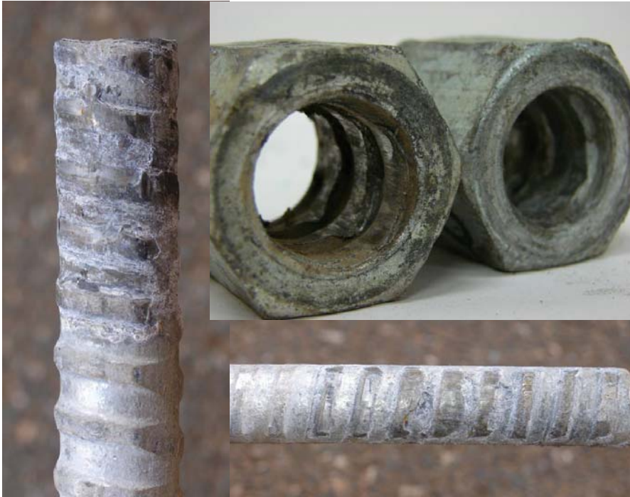
Figure 12. Thread stripping on the nut and bar.
