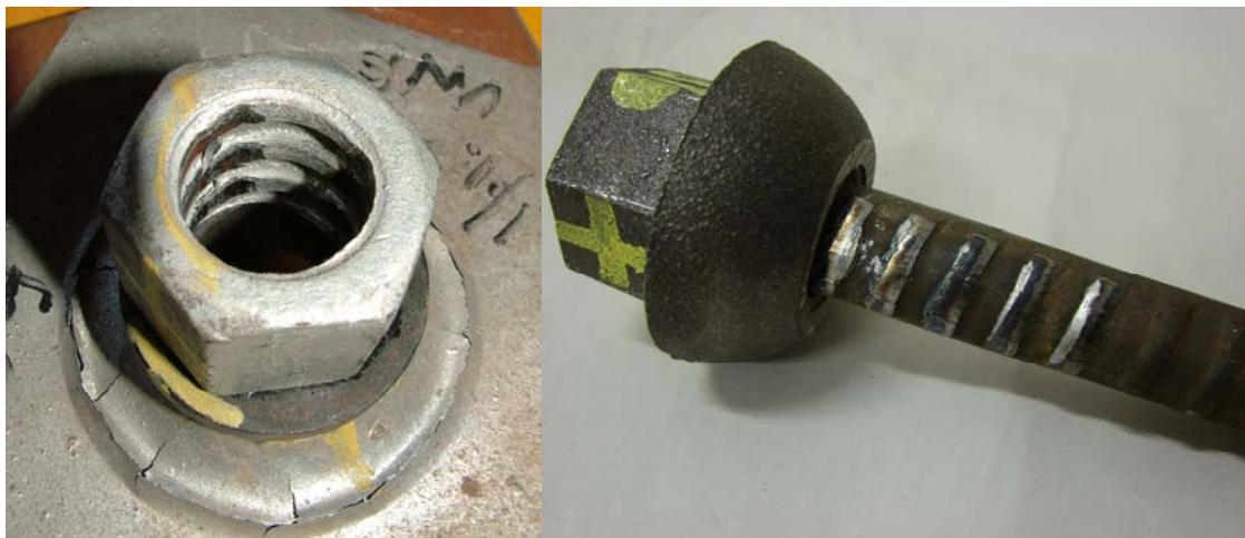
Figure 11 : Debonded threadbar results - stripped nut and stripped thread
