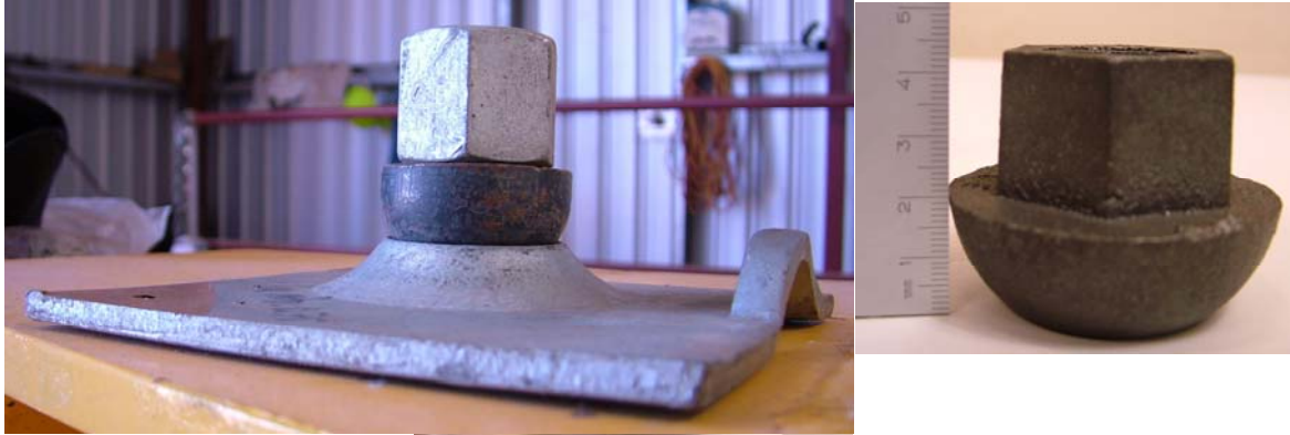
Figure 9: Separate nut and washer and the integrated nut and washer
