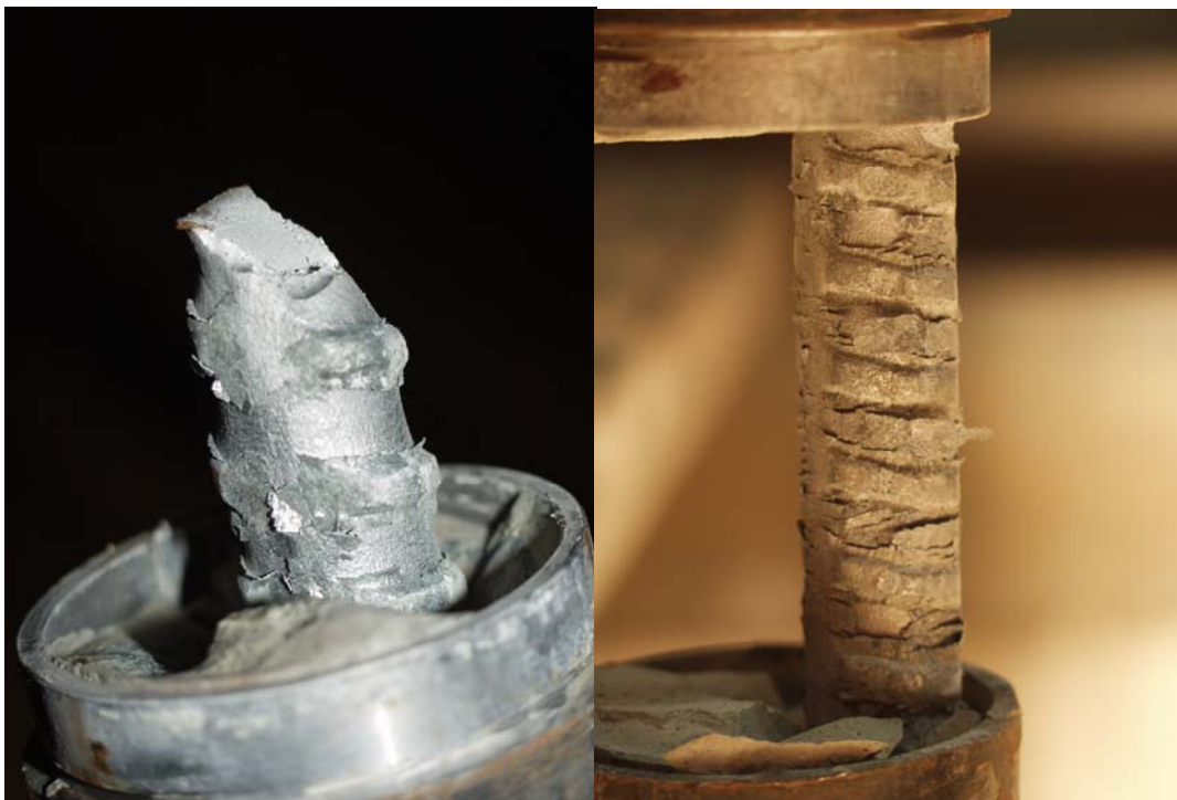
Figure 7 : Threadbar results – snapped first loading and yield first loading
