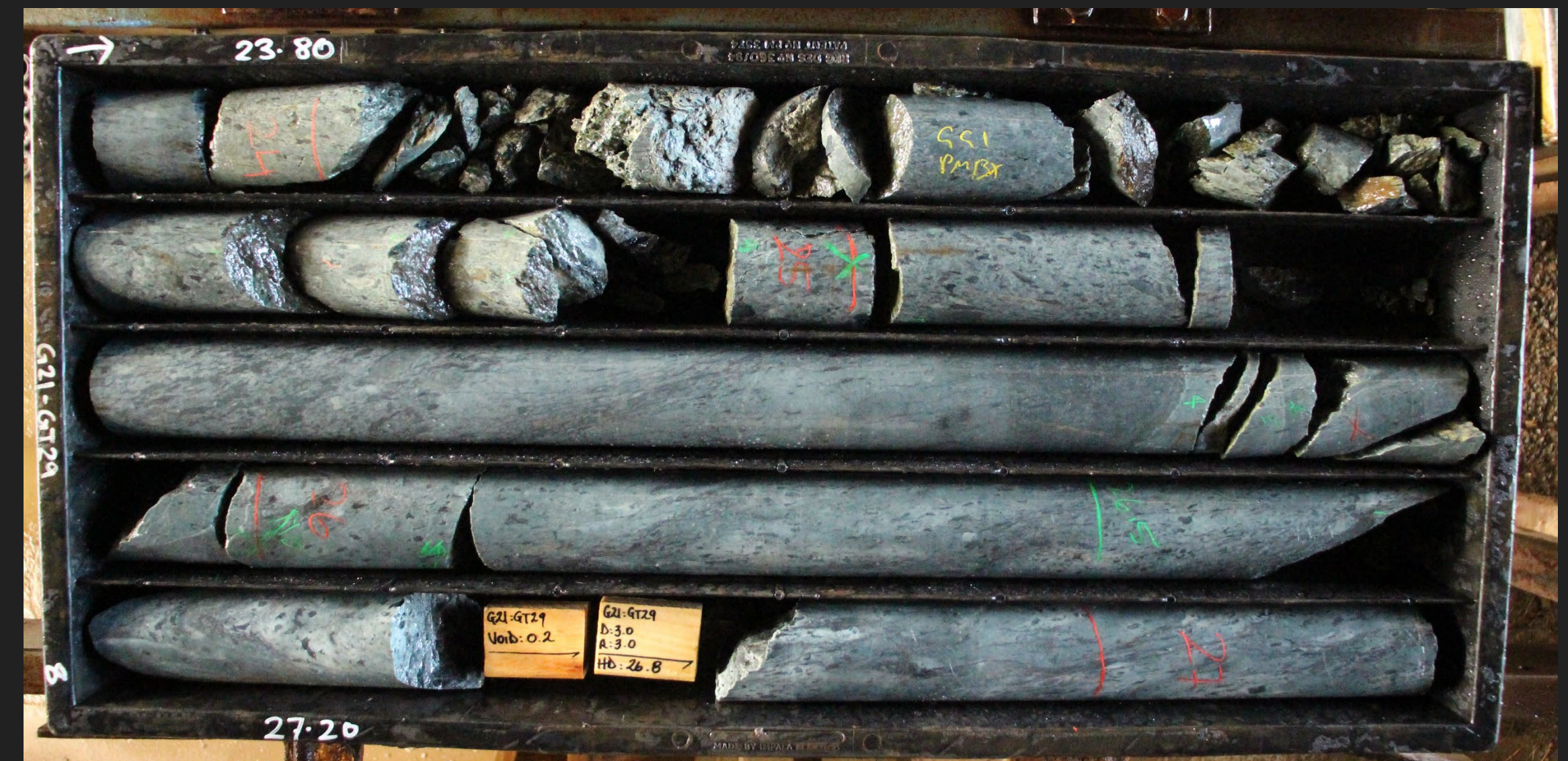
Water loss on fault
