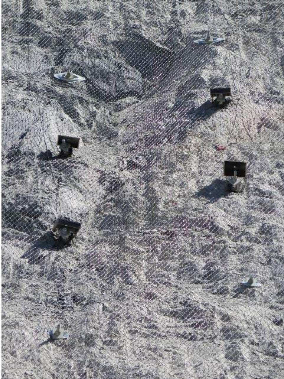
FIG 13 – Mesh tensioned with spike plates and load cells measuring bolt collar load.
